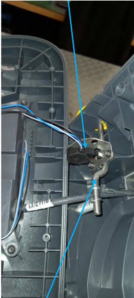
Actuating bracket connected With rotary handle (yellow)
